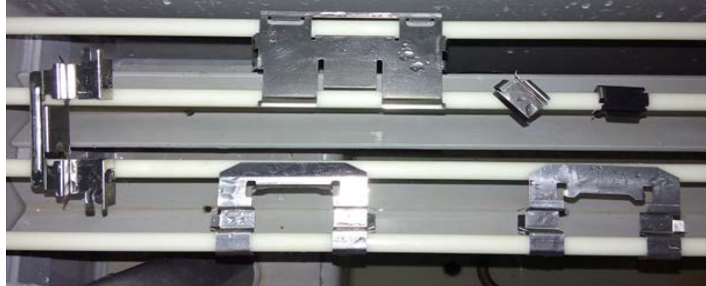
301 Stainless after 200 hrs. Salt Spray
