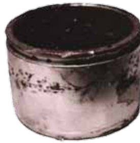
Rust in the caliper bore or on the piston prevents the caliper from releasing from the rotor, resulting in excessive heat
