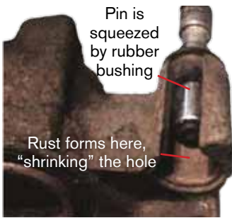
Rust on the caliper housing "squeezes" the bushings or pins causing the caliper housing to "freeze" and not move.
