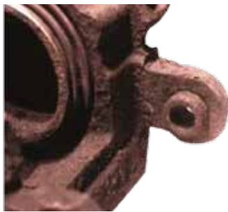
Rust on the caliper and/or bushings prevents free movement.
