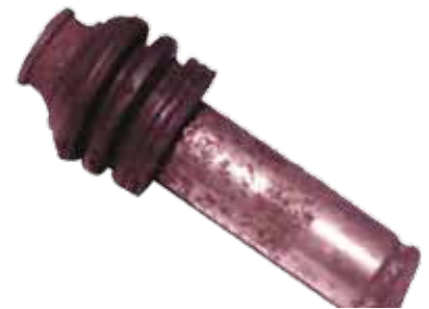
No lubrication on bushings and/or pins prevents free movement
