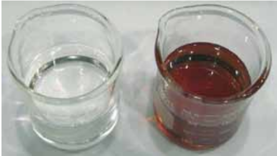
Actual Beck/Arnley ATF base oil (left) compared to typical aftermarket ATF base oil (right).
